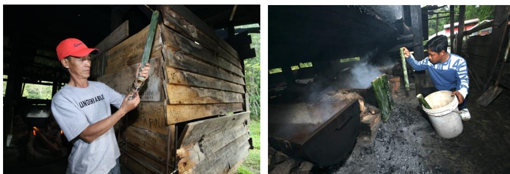
Figure 5: A small hole is drilled in the bottom of the bamboo to remove excess brine before it is dried again on the edge of the embers.
