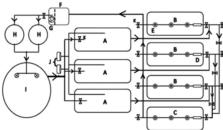
**Figure 1.** Top view of ARS. A: Culture tank, B: hydroponics trough (planted bed), C: hydroponics trough (control bed), D: filter, E: sprinkler, F: sump, G: pump, H: rapid sand filter, I: water storage tank, J: air blower, and K: valves.
