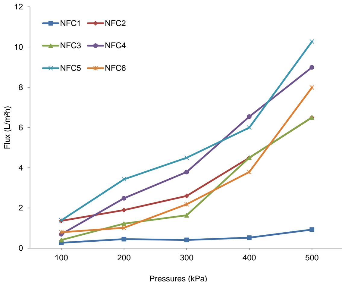
Figure 3. PWP of nanofiltration membrane at different pressure.
