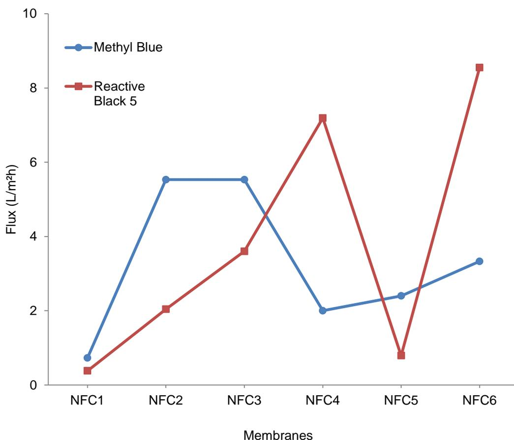
Figure 4. Dyes flux with different concentration of CTAB.
