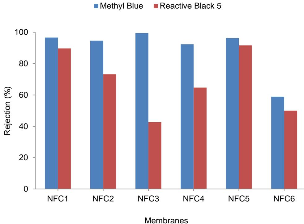
Figure 5. Dyes removal of NF membrane with concentration of CTAB.
