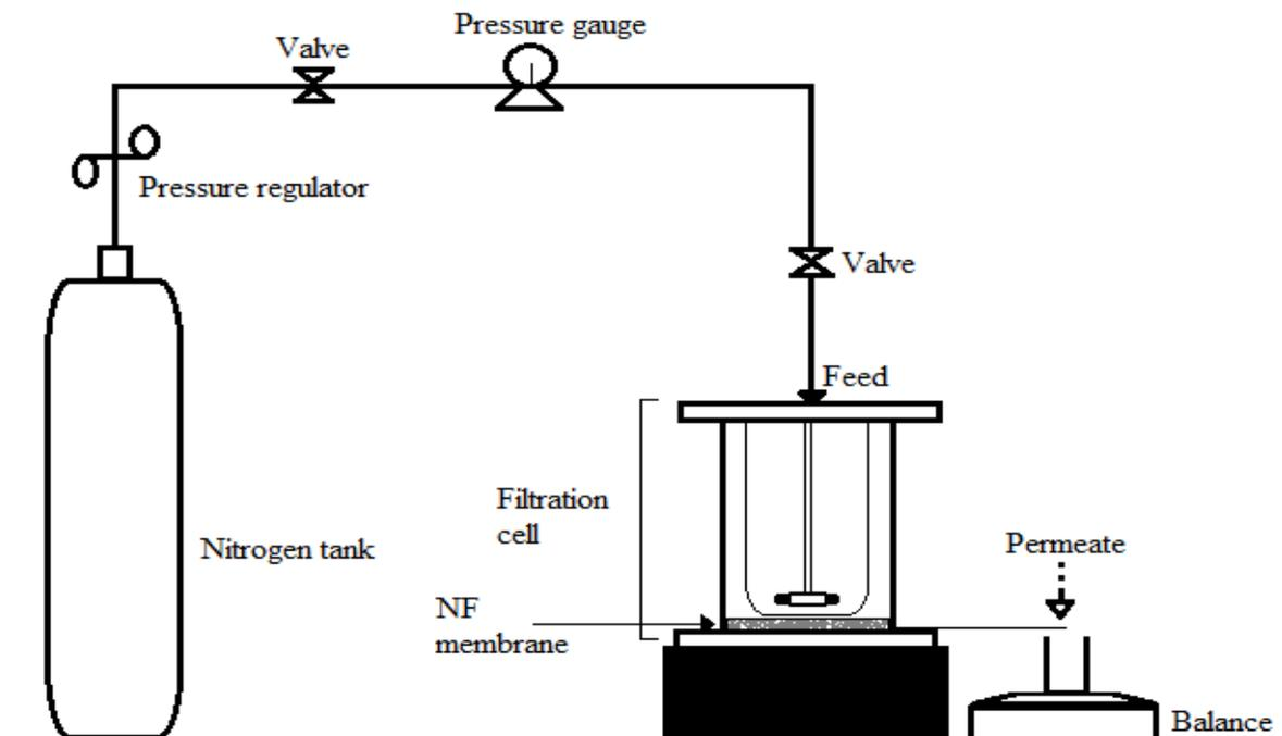
Figure 2. Nanofiltration set up.
